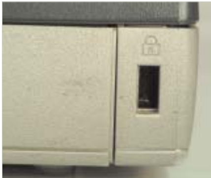
The security slot will keep your laptop where you last left it
